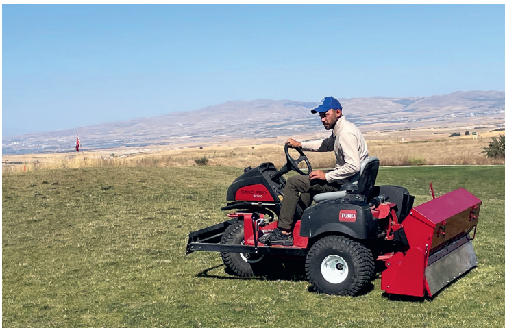
The STAR-Seeder can be short-coupled with a bunker-vehicle.
