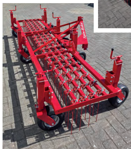
Spin-Rake 300 Short Version (4 rows of tines only) with foldable wings follows undulated golf fairways nicely.
