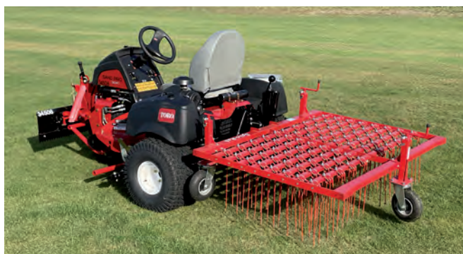
Spin-Rake model 150 with special A-frame hitch fitting Toro Sand Pro bunker rake.
