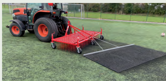
The Spin-Rake loosens the infill in synthetic turf pitches.
