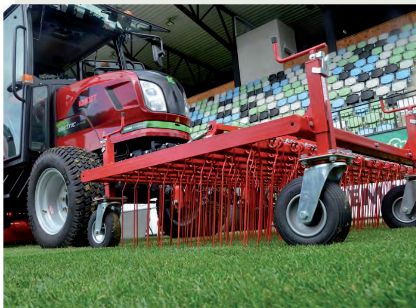
Spin-Rake 6m with Trilo vacuum cleaner in the rear.
